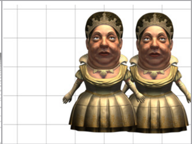
The distance does not affect the size of the item. ( Orthographic mode)
